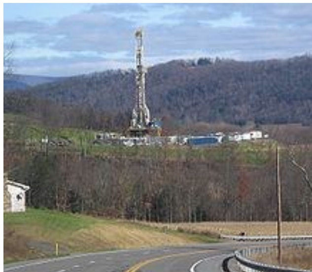
Horizontal drilling rig for natural gas in the Marcellus formation in eastern Lycoming County, Pennsylvania
